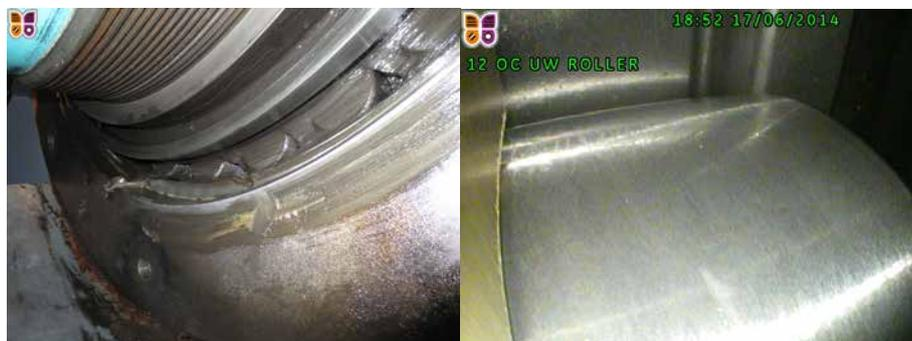
*Bearing in as found condition (left) and after flushing to remove grease (right)*
