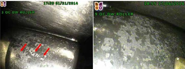
*Micropitting and debris denting on the roller at first flush (left) and 5 months later (right) damage progression has slowed*
