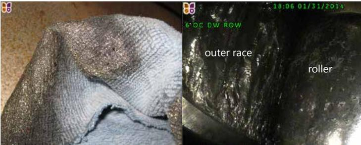
*Debris evident in original flush grease (left), outer race condition before first flush (right) showing severe spalling*
