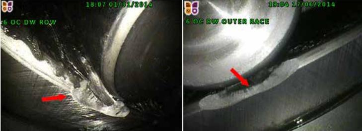
*Outer race fracture after first flush (left) and 5 months later (right), showing damage progression has slowed*
