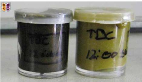
*Typical samples showing condition of grease before flushing (left) and improved quality 5 or more months after flushing (right)*
