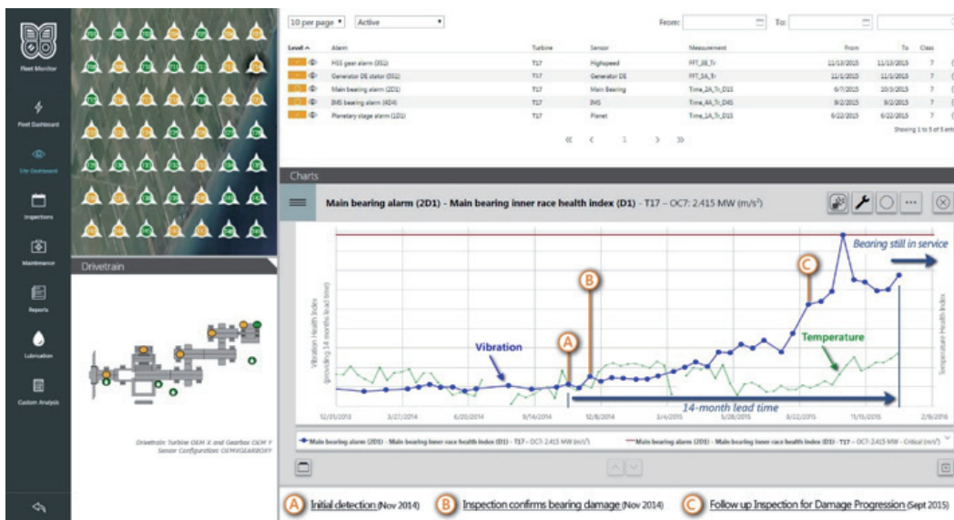
Figure 6 – Romax Fleet Monitor™ providing over 14 months warning on main bearing damage. First detection at Point A. Inspection at Point B confirming significant spalling on the raceways and rollers. Re-inspected at Point C after monitoring engineers warn of recent rise in the health index.
