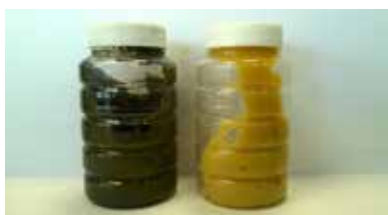
Grease extracted before (left) and after (right) a grease flushing campaign
